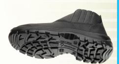
Sole: Made of two layers of polyurethane, directly injected in the upper; softer and lighter midsole (first layer) - density 0,4g/cm³, providing more comfort; and more compact sole (second layer) – density 0,9g/cm³, sharp objects and abrasion resistant with antislip system made up of special grooves, 3mm height, 6mm width and resistant to slipping on ceramic and steel floors (SRC Level).
