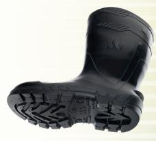
Note: Class II insulating footwear has the purpose of insulation in small repairs and low voltage electrical installations. Class OO: Usage maximum voltage: 500V (CA) or 750 (CC).
